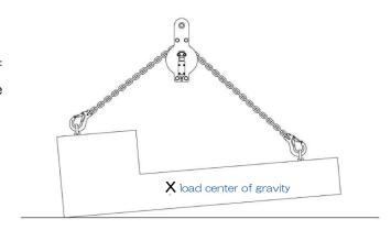
4. To adjust the balance, move the BALANCE MASTER over the center of gravity while the chain is moving freely.
