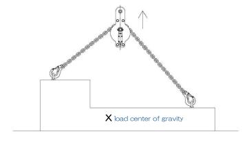
3. If only one side is lifted, it means the center of gravity has shifted. Stop lifting and lower the load.
