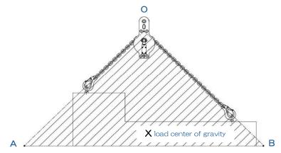
Lift with an angle within 90°. Also, make sure that each leg angle is 60° or less.
